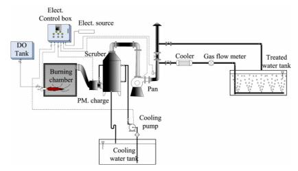
Figure 4. Experimental ballast water treatment system using inert gas
