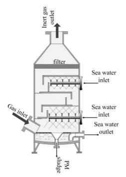
Figure 2. Electrostatic filter water tower
